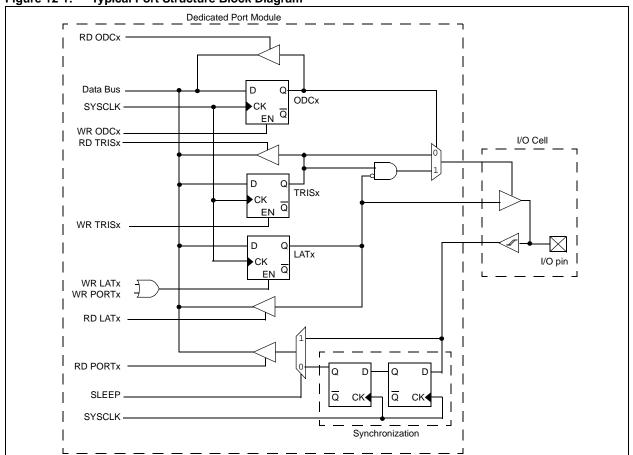
Figure 12-1: Typical Port Structure Block Diagram
